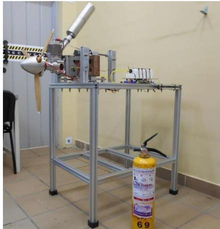
*Figura 3 USB Propeller Testing Bench (Rojas Mora, Cano Bernal, & Mónico Muñoz, 2018)*
