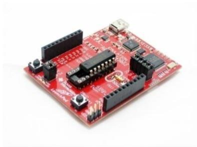
*Figura9.* Placa TI MSP30 de Texas Instruments.
