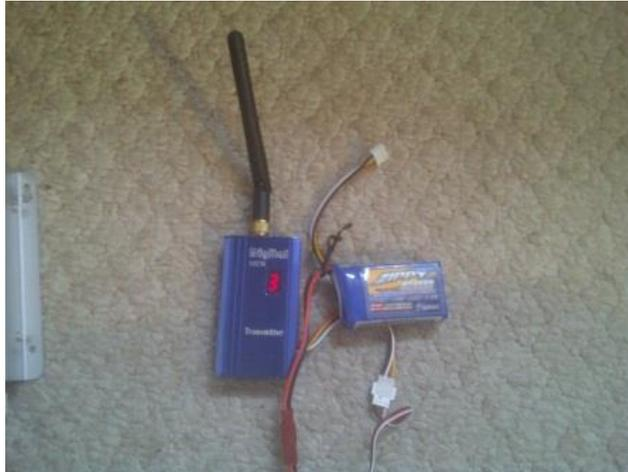
Figura 35. **TRANSMISOR DE LA VIDEO-CÁMARA**
